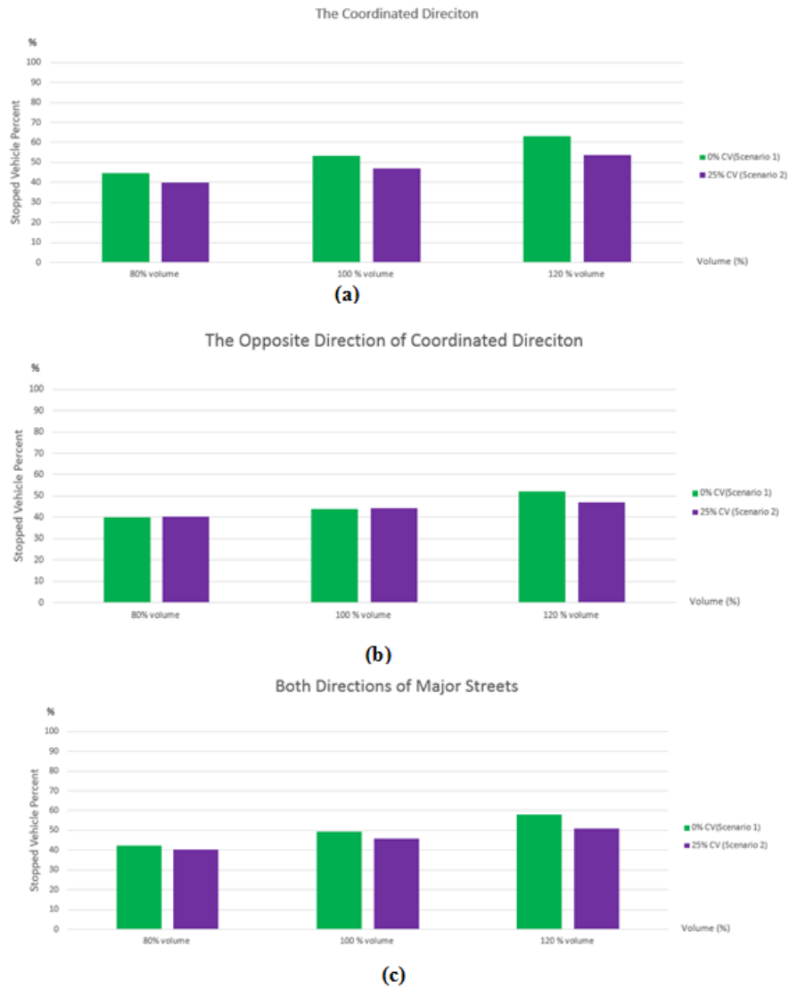
Figure 4.14 Stopped Vehicle Percent of the Study Arterial under Volume Variations
